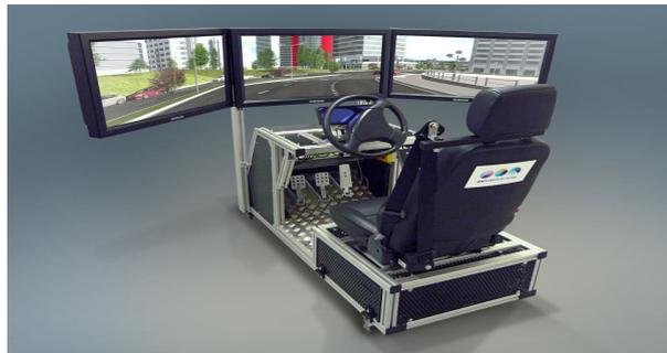
Figure 2.22: SCANer™ studio compact simulator setup.
