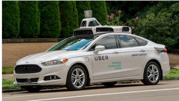
Figure 2.3: Ford Fusion Uber ATC car (Uber Advanced Technologies Group 2018).[13]
